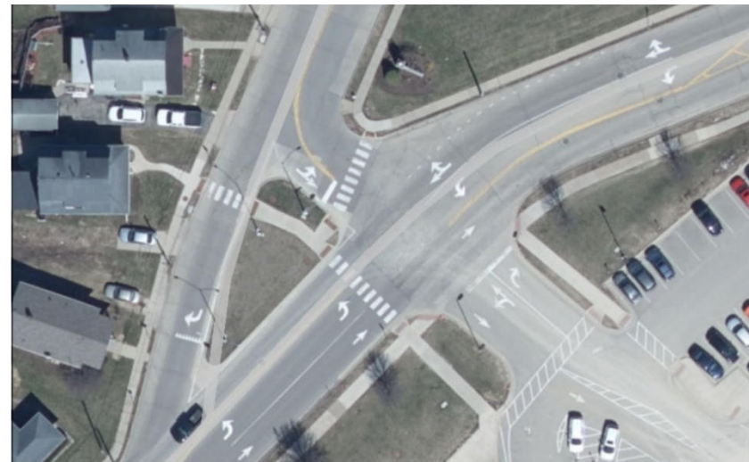
Pedestrian refuge island outside Dubuque Senior High School (Source: ECIA using Dubuque County GIS)
